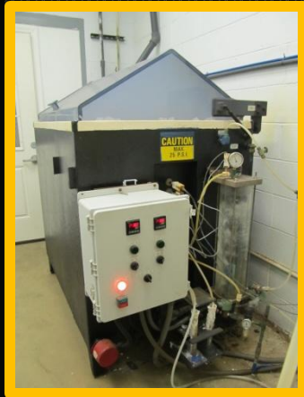
AutoTech 36x42 Salt Spray Cabinet, Testing per ASTM B117 Spec
